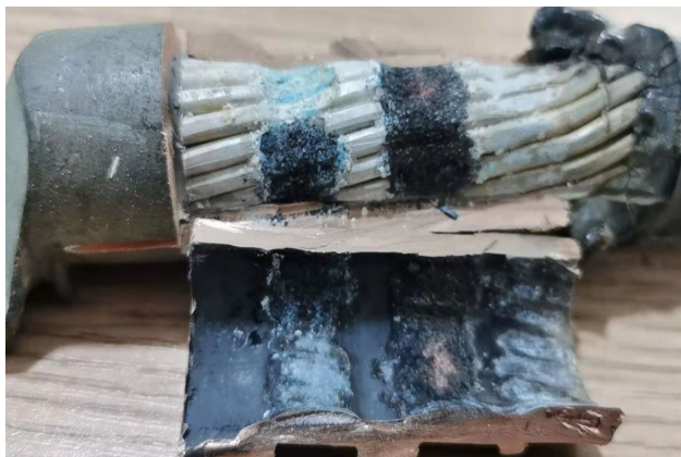
图 5 铜镀锡线夹发热故障
